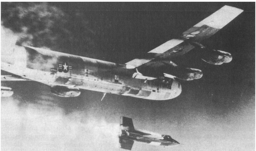
Figure 16 X-15 rocket research aircraft shown just after its release from a Boeing B-52 aircraft. The X-15 shown is one of the early models, fitted with interim XLR-11 rocket engines (ca. 1960, NASA photo 60-X-38).
