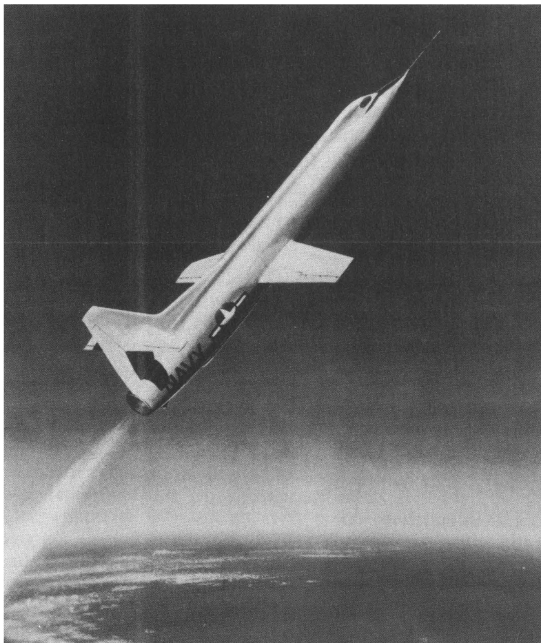
Figure 11 Artist's concept of the Douglas D-558-3 hypersonic aircraft which remained a paper study. Douglas Aircraft Co. photo.
