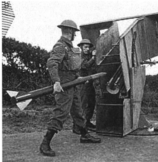
Figure 10–13: A 3 inch UP being loaded onto an early single barrel projector. The final rockets were some 76 inches long with shell, 3.25 inches diameter and weighed some 50 pounds.
