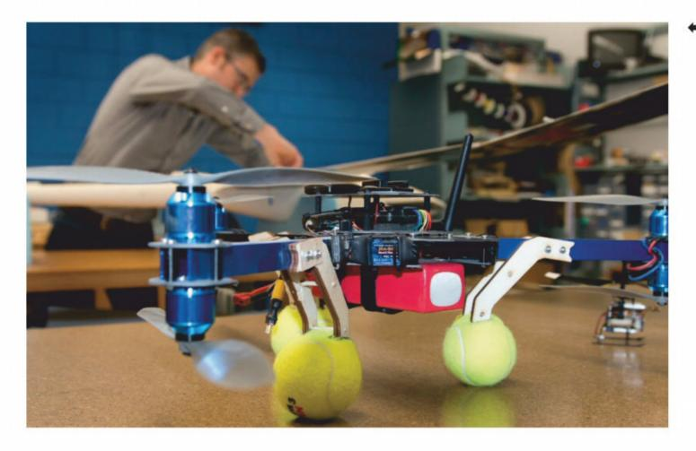
Like this tiny drone at Jack Langelaan's Penn State lab, Dragonfly will have counter-rotating rotors, one atop the other. Only recently has drone technology advanced enough to make Dragonfly possible.
