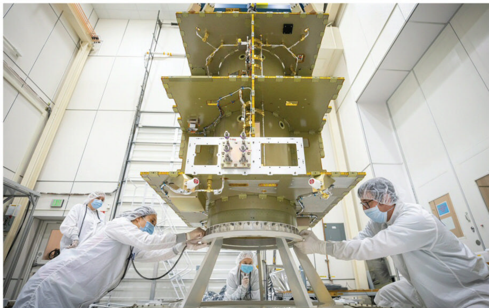
➔ The DART team installs electrical subsystems in APL’s clean room. DART has little in terms of electronics—it is mostly a mass demonstrator—but what it does have is cutting-edge.
