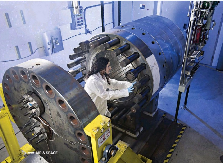
← The 800-liter GEER pressure chamber at NASA's Glenn Research Center in Cleveland, Ohio, duplicates the temperature, pressure, and chemistry of the Venus atmosphere.
