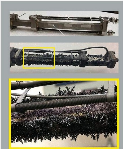
↑ In the Glenn Extreme Environment Rig (GEER), an aluminum waveguide was exposed to sulfur dioxide and other components of the Venus atmosphere. It reacted badly.
