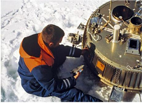
A scale model of the Huygens probe rests in the snow after surviving a drop test from a height of 24 miles (38 km) to make sure its protective shields would separate and the parachute release system would deploy as expected on Titan. ESA
