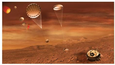
After entering Titan's atmosphere, the Huygens probe deployed a parachute to slow its descent, eventually ejecting its protective outer shell and exposing its instruments. The probe took measurements of the atmosphere and imaged the world around it, continuing to beam back data from its landing site for over an hour. ESA-C. CARREAU
