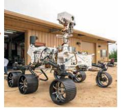
On September 4, while Perseverance was en route to Mars, JPL moved the rover's twin — a full-scale engineering model dubbed OPTIMISM (Operational Perseverance Twin for Integration of Mechanisms and Instruments Sent to Mars) — to its "Mars Yard" test area. Engineers can test rover commands and operations using OPTIMISM in an environment that simulates the Red Planet to better understand what Perseverance is experiencing on Mars. NASAUPL-CALTECH
