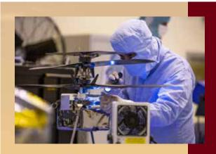
The experimental helicopter drone Ingenuity will become the first aircraft to take powered flight on another world. Though it won't be able to wander far — it will stay less than 0.6 mile (1 km) from the Perseverance rover to remain in wireless communication (right) future drones could serve as more capable scouts. At left, Ingenuity receives its final inspection at the Kennedy Space Center in Florida before being mounted to Perseverance for its journey to Mars. NASAJIPL-CALTECH
