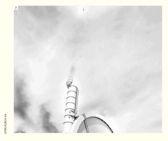
1 The team plans to fit the three-metre-long rockets launched by the L100 (shown here in a CGI render) with internal boosters that kick in when they reach the upper atmosphere, allowing them to be manoeuvred into the desired position.
