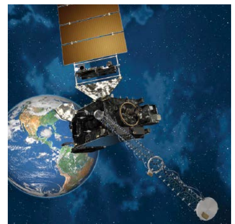
The first weather satellite in the GOES-R series, now designated GOES-16, observes Earth from geostationary orbit in this artist's rendering. The satellite became fully operational in December 2017. Credit: NOAA/Lockheed Martin
