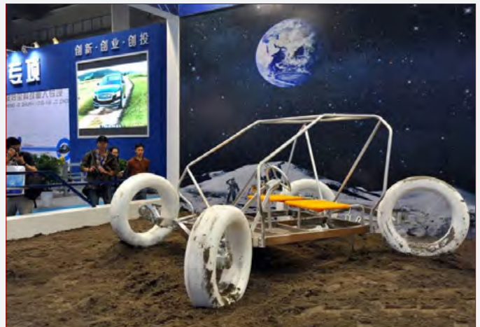
The manned lunar rover, developed by a joint team of the Ministry of Education, displayed in an exhibition. It adopted a foldable design. (credit: Chinese internet)
