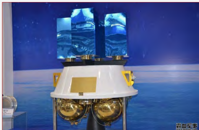
China is developing the first liquid-fuelled general upper stage called Yuanzheng 1 but no picture of it is available. Here is the scale model of the Advanced Upper Stage, the next generation upper stage after Yuanzheng 1 (Expedition 1). (credit: Chinese internet)
