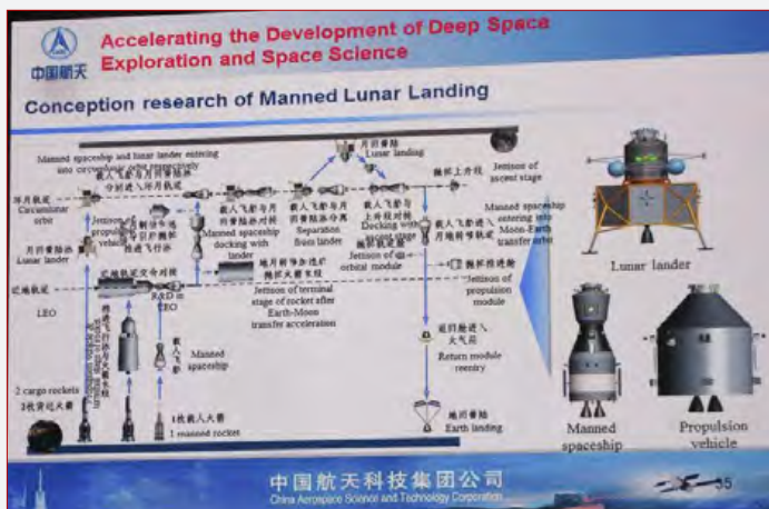
The PPT slide showing the Chinese manned lunar landing mission profile in IAC 2013. (credit: CASC/Go Taikonauts!)
