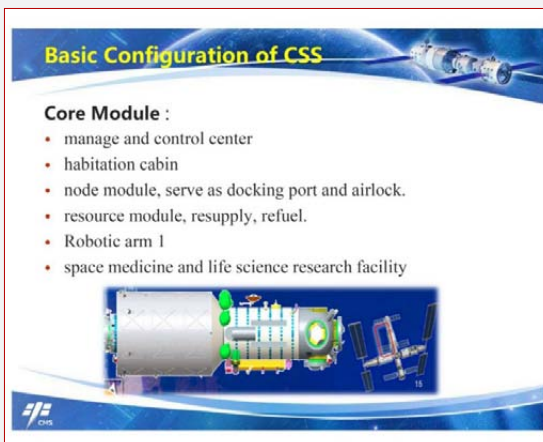
Graphic and basic function of the Core Module of the future CSS. (credit: Ji QiMing/CMSA)
