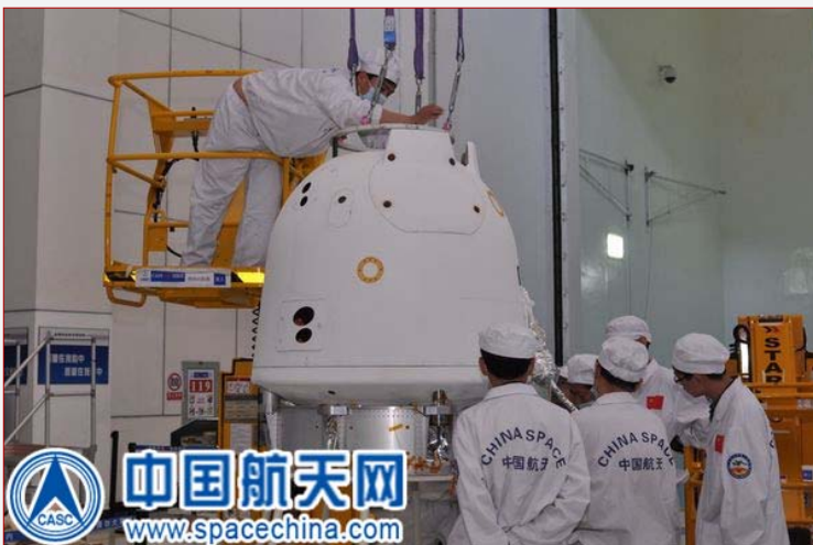
Re-entry capsule of the Chang'e 5 Pathfinder mission. (credit: spacechina.com)
