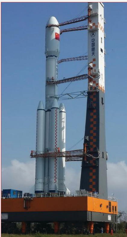
left: CZ-7 at the mobile launch platform in rehearsal in Wenchang Space Launch Centre (credit: Chinese internet)
