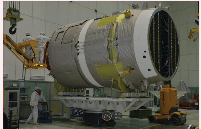
Tianzhou 1 cargo vehicle in testing. An open window at the unpressurised section is seen at the top. (credit: China Space News)
