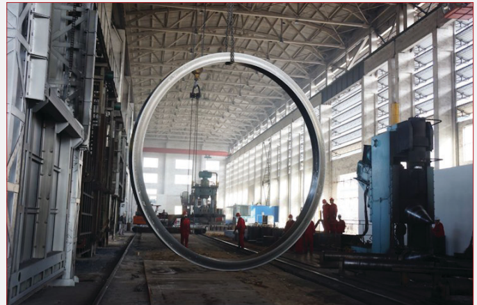
One of the large diameter rings required by CZ-9. (credit: China Space News)
