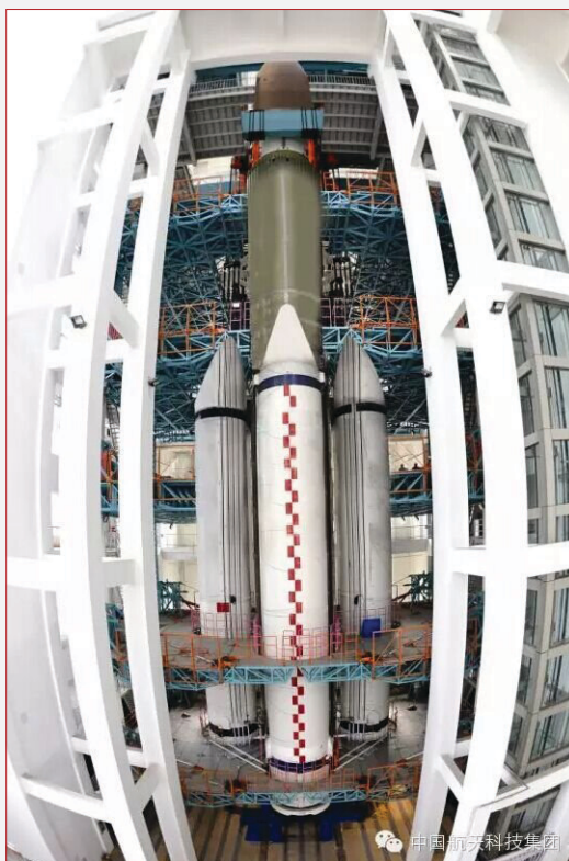
right: A CZ-5 completed assembly in Tianjin. (credit: CASC)
