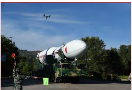
CZ-6 and its erector on the transportation vehicle. The picture was taken during the rolling out. (credit: SAST)
