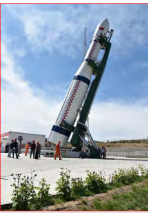
CZ-6 being erected at the launch pad. (credit: SAST)
