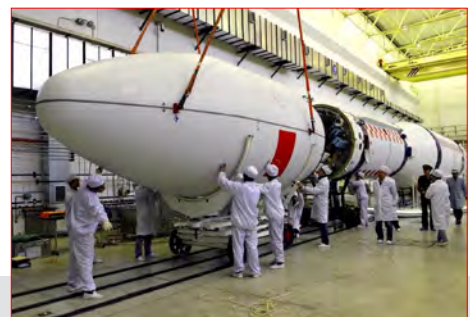
CZ-6 in rocket - satellite horizontal mating. This was the flight model launched on 20 September. Note that all follow-up images show the flight model. (credit: SAST)
