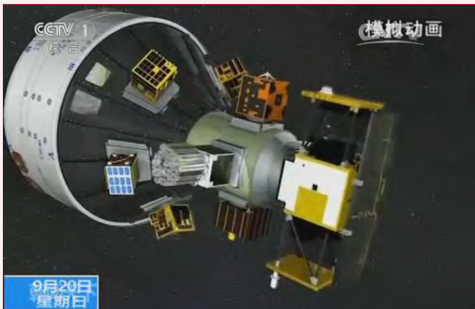
The 20 small and micro satellites attached on the CZ-6 adapter. (credit: CCTV)
