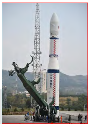
CZ-6 sitting at the launch pad. The erector was partially put down. (credit: SAST)
