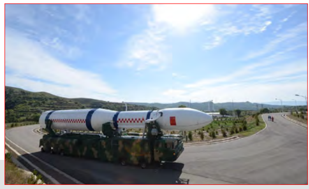
CZ-6 and its erector on the transportation vehicle. The picture was taken during the rolling out. (credit: SAST)
