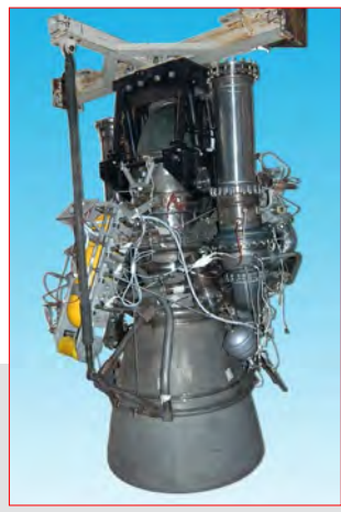
The YF-100 engine. A single YF-100 is used on the first stage of CZ-6. (credit: Chinese internet)
