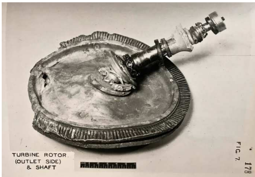
■ A contemporary image of a recovered turbine rotor and shaft.
