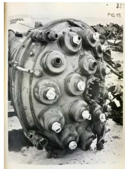
■ A contemporary image of a recovered combustion chamber showing the burner cups around the central oxygen inlet.
