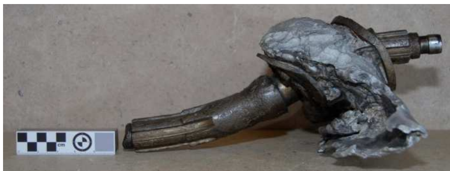
■ The conserved turbo-pump shaft and remains of rotor disc from the Marden V2.
