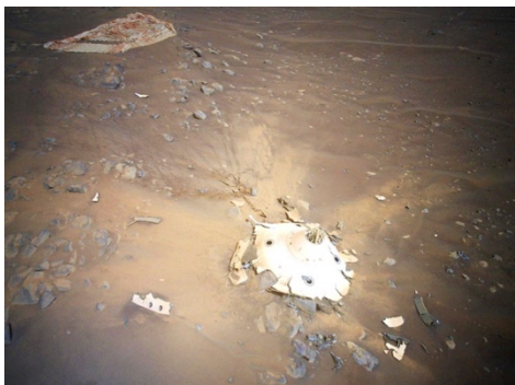
Fig. 2. Helicopter color camera image of the backshell and parachute on the edge of north Séítah acquired on flight 26 (the next flight after the longest flight across north Séítah). Note radial blast pattern around backshell.
