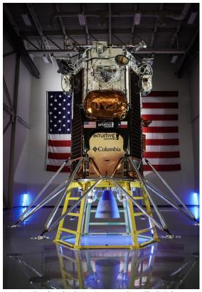
Figure 1: The finished IM-1 Nova C, called Odysseus, just prior to shipping to KSC for launch. The Nova-C is capable of delivering more than 130 kg of payload to anywhere on the Moon
