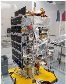
Figure 2: IM hopper. Approximately 1 meter tall, and capable of flying 8 kg of payload more than 25 km.
