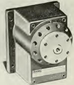
Basic unit consists of a stator having 12 input ports and a rotor that connects any one of these to an output port. A unidirectional high-torque motor rotates the rotor to a desired position and built in provisions are available for indication of position either visually or digitally for operation of recording devices.
