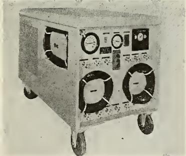
The ACE-37 cart is rated for 3,000 psi pressures, has a capacity of 18,000 cu. in. and weighs about 2,000 lbs. It measures 42" high, 38" wide and 60" long.
