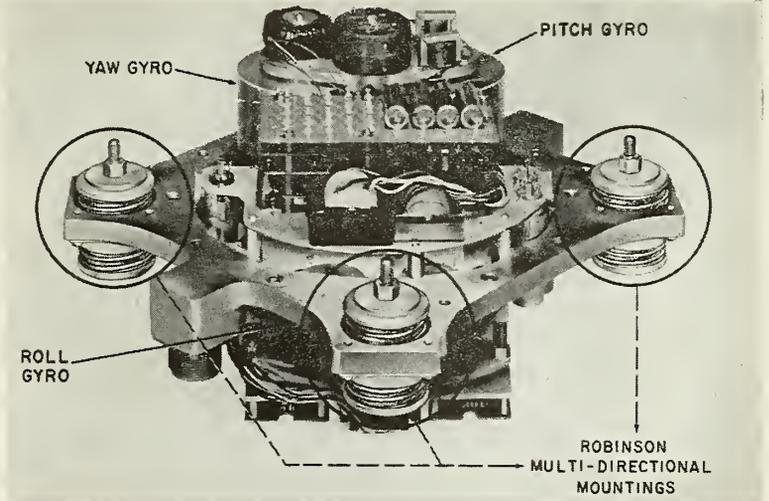
Multi-directional mounting system built by Robinson Aviation, Inc. will protect Vanguard earth satellite's Minneapolis-Honeywell inertial guidance system. Four Robinson Met-L-Flex resilient elements will be attached to the rocket bulkhead with the equipment installed inside. Mounting system is designed to instantly attenuate shock of 6 g or vibration over 65 cps.
