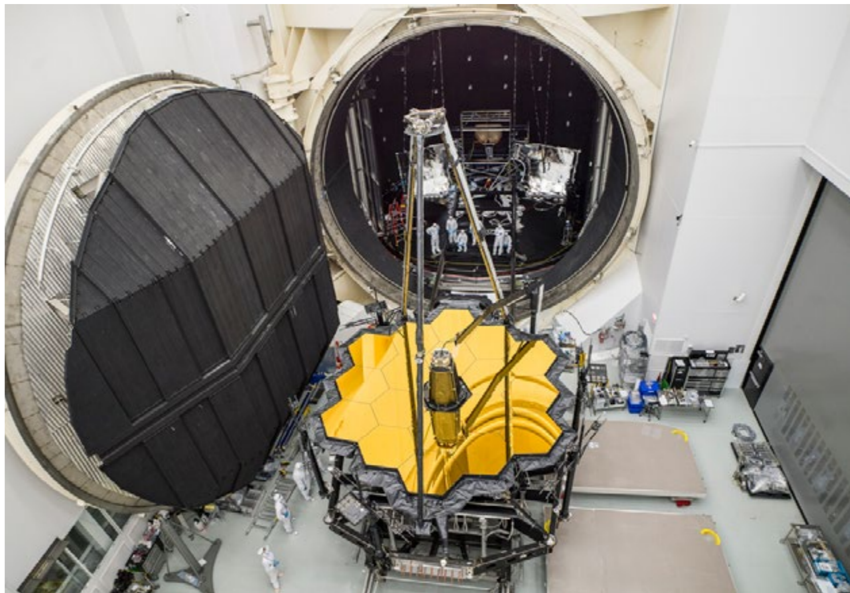
The James Webb Space Telescope’s scientific instruments and optical elements—including its gold-plated 6.5-meter primary mirror—emerge from cryogenic testing at NASA’s Johnson Space Center in Houston on December 1, 2017.
