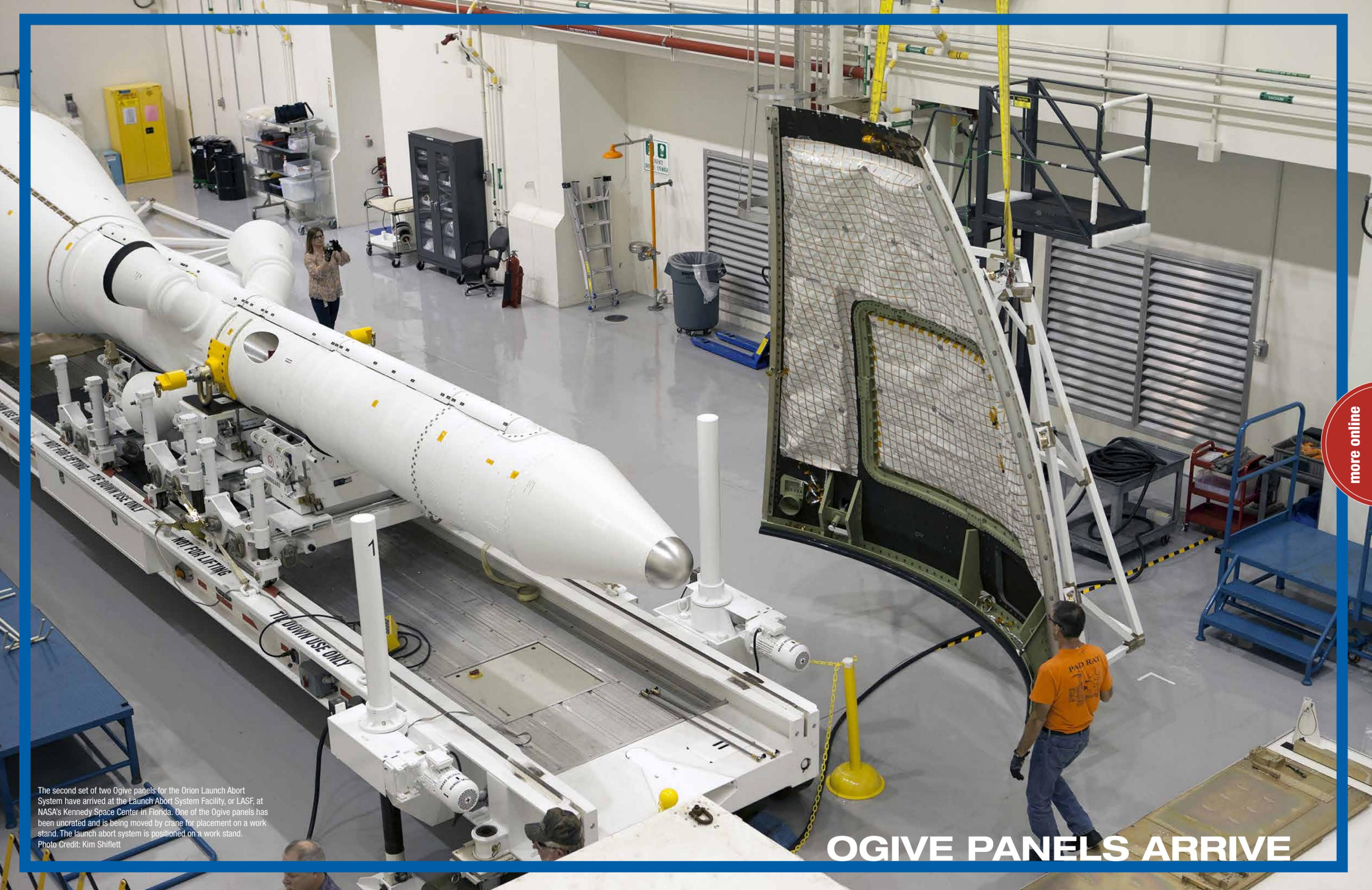
The second set of two Ogive panels for the Orion Launch Abort System have arrived at the Launch Abort System Facility, or LASF, at NASA's Kennedy Space Center in Florida. One of the Ogive panels has been uncrated and is being moved by crane for placement on a work stand. The launch abort system is positioned on a work stand. Photo Credit: Kim Shiflett
