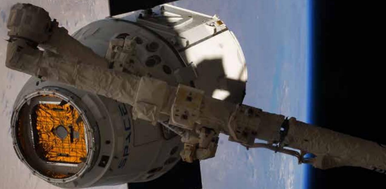
A SpaceX Dragon spacecraft full of cargo, experiments and equipment blazed into orbit Friday, April 18, on the strength of one of the company's Falcon 9 boosters. Two days later, the Dragon arrived at the International Space Station where it was grappled by the Canadarm2 and locked into place so astronauts could later retrieve almost 5,000 pounds of equipment, experiments and supplies.
