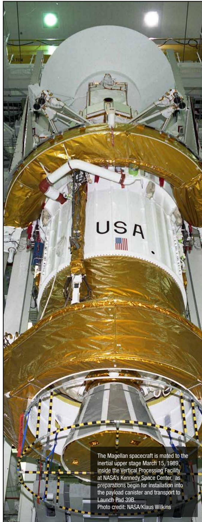
The Magellan spacecraft is mated to the inertial upper stage March 15, 1989, inside the Vertical Processing Facility at NASA's Kennedy Space Center, as preparations begin for installation into the payload canister and transport to Launch Pad 39B. Photo credit: NASA/Klaus Wilkins
