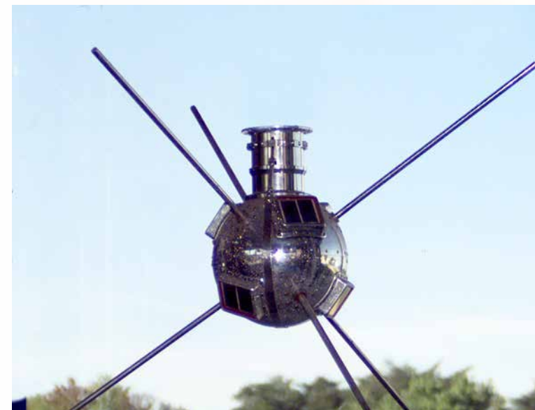
Launched March 17, 1958, Vanguard 1 was America's second Earth satellite and was the first powered by solar cells. It was designed to test the launch capabilities of the three-stage Vanguard rocket and the effects on satellite systems in orbit. Photo credit: NASA
