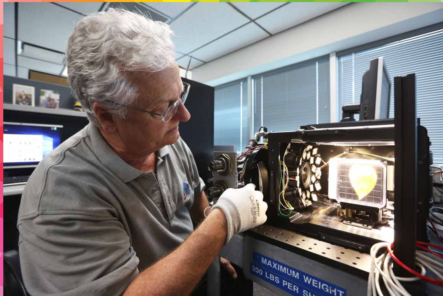
Dr. Scott Shipley of Ascentech Enterprises makes an adjustment to the Spectrum unit. He is the project engineer for the effort working under the Engineering Services Contract at NASA's Kennedy Space Center. The device is being built for use aboard the International Space Station and is designed to expose different organisms to different colors of fluorescent light while a camera records what's happening with time-lapse imagery. Results from the Spectrum project will shed light on which living things are best suited for long-duration flights into deep space. Photo credit: NASA/Cory Huston
