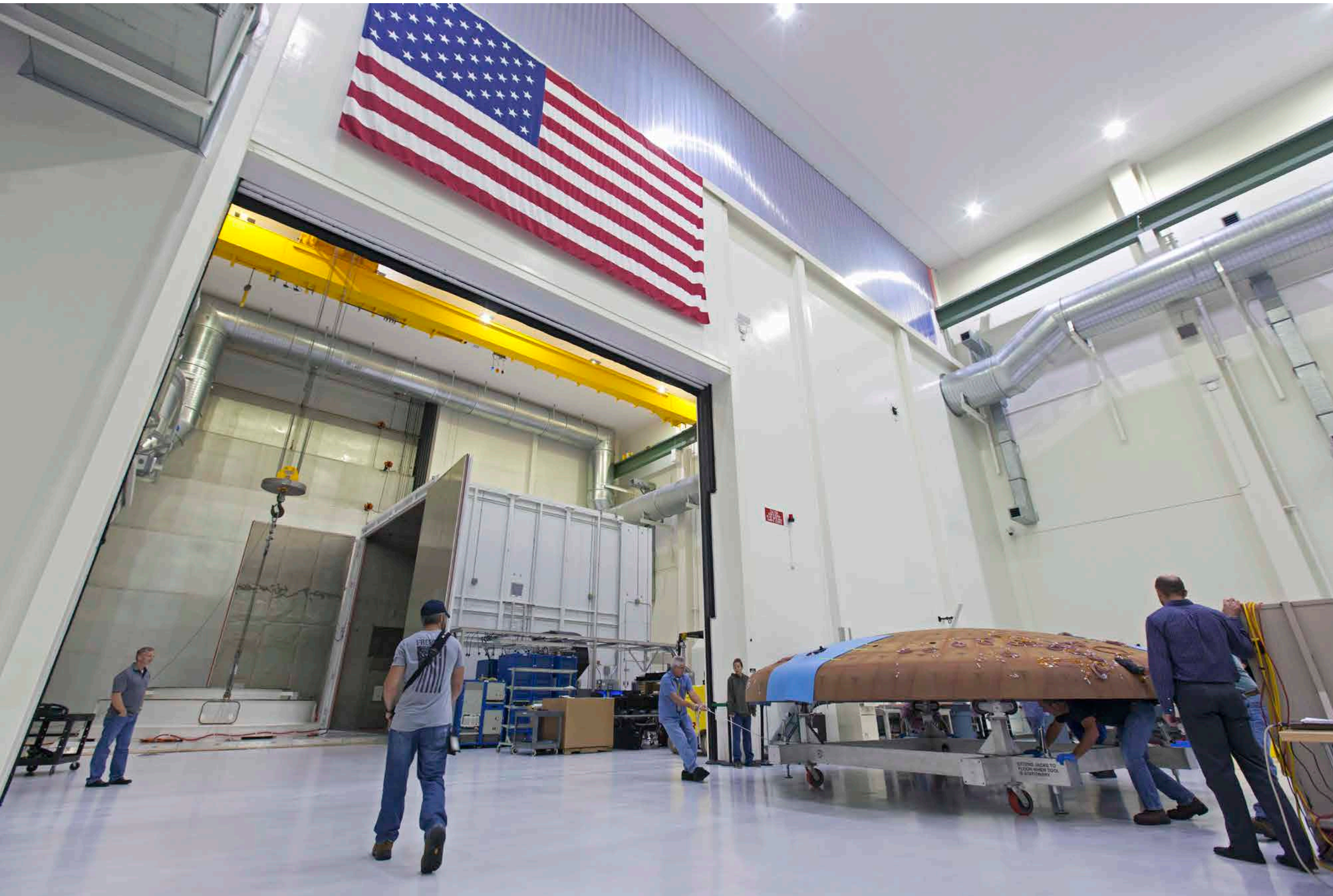
Technicians move the Orion heat shield for Exploration Mission-1 toward the thermal chamber in the Neil Armstrong Operations and Checkout Building high bay Oct. 23, 2017, at NASA's Kennedy Space Center. Protective pads have been attached to the heat shield surface. The heat shield will undergo a thermal cycle test to verify acceptable workmanship and material quality. The test also serves to verify the heat shield's thermal protection systems have been manufactured and assembled correctly. The Orion spacecraft will launch atop NASA's Space Launch System rocket on its first uncrewed integrated flight, Exploration Mission-1. Photo credit: NASA/Ben Smegelsky
