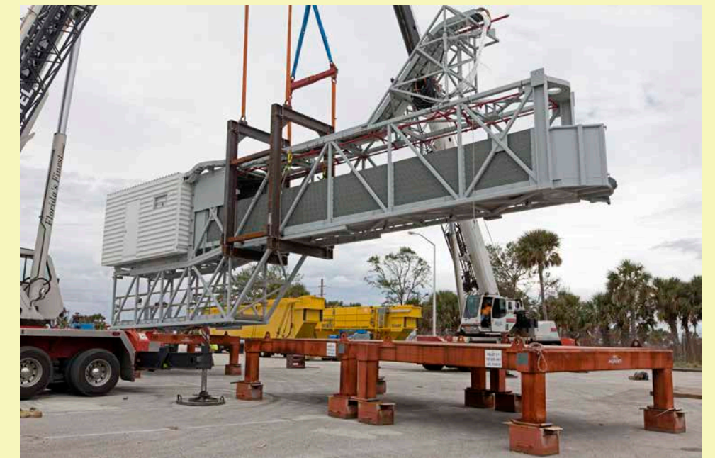
The Orion crew access arm is moved by crane onto a flatbed truck at Precision Fabricating and Cleaning in Cocoa, Florida, on Oct. 16, 2017, for the trip to NASA's Kennedy Space Center. Photo credit: NASA/Kim Shiflett
