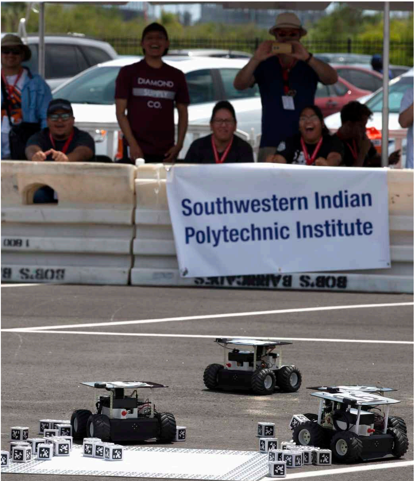
During the final round of the Swarmathon competition at the Kennedy Space Center Visitor Complex, students from Southwestern Indian Polytechnic Institute (SIPI) in Albuquerque, New Mexico, watch their robots as they look for cubes identified by their AprilTags, similar to a barcodes. The Swarmies were programmed to deliver the cubes to a “home” square in the middle of a competition arena. SIPI captured first place in the competition winning a $5,000 cash prize. Photo credit: NASA/Kim Shiflett
