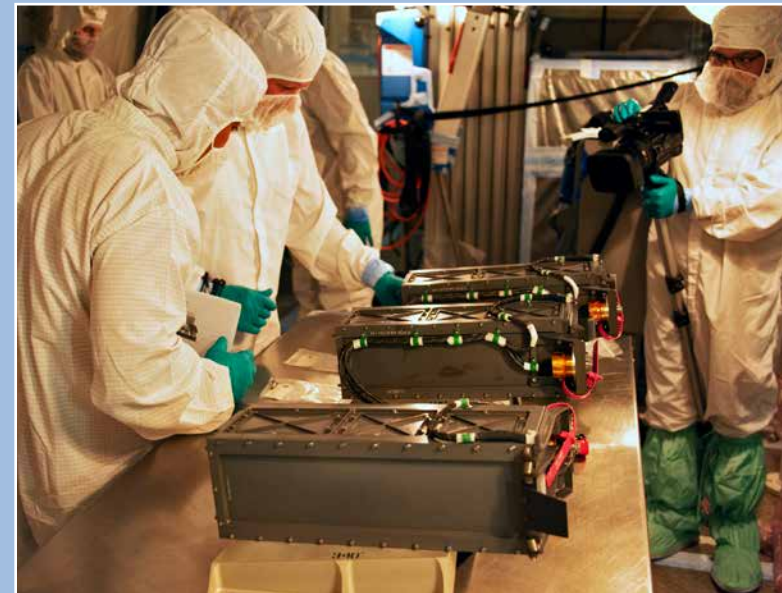
(Above) At Space Launch Complex 2 at Vandenberg Air Force Base in California, technicians prepare three poly picosatellite orbital deployers, or P-POD containers, with tiny satellites, called CubeSats inside, for installation on the second stage of the United Launch Alliance Delta II rocket, on Aug. 31, 2018. Photo credit: USAF 30th Space Wing/Julio Paz
