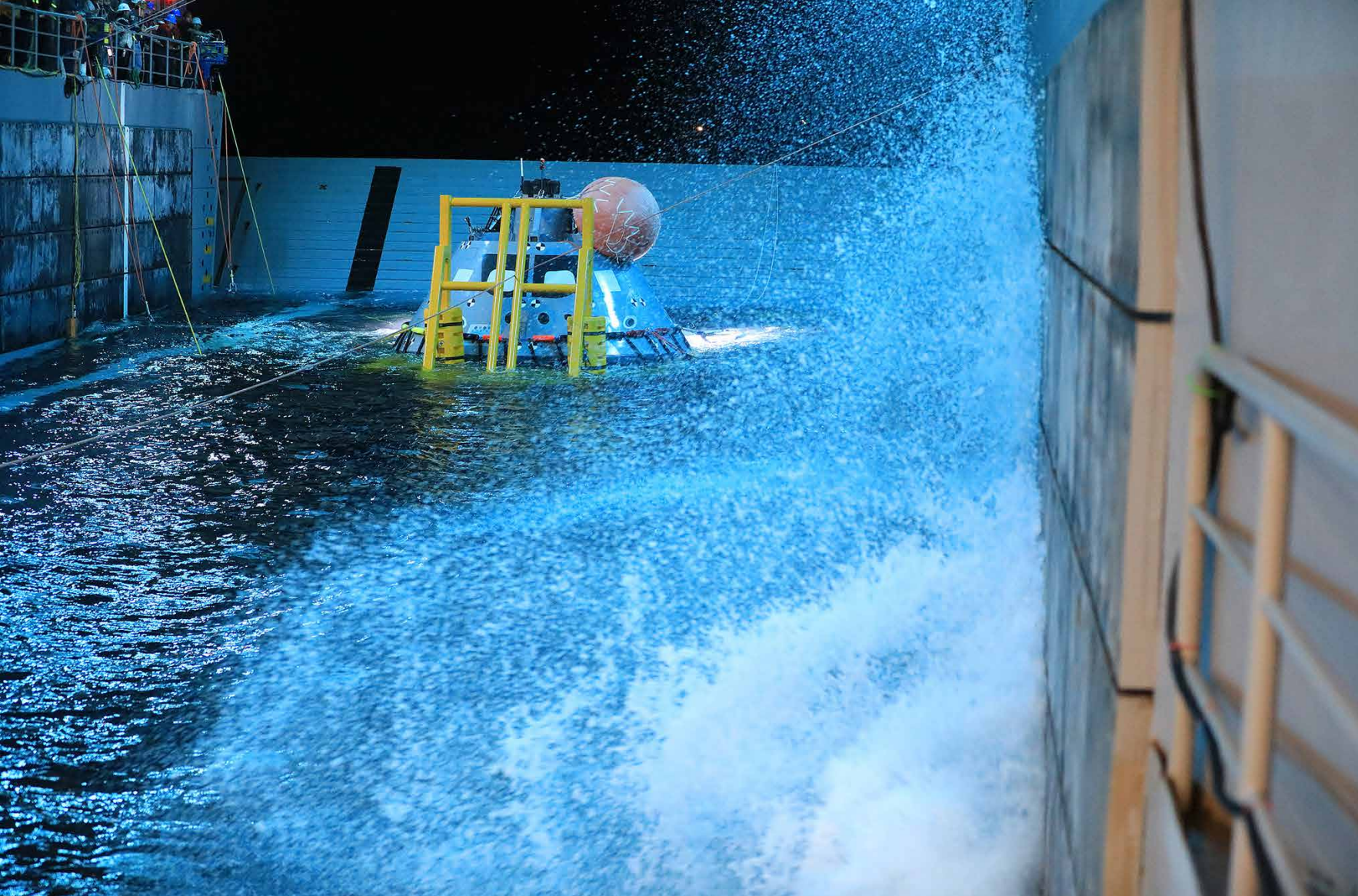
A test version of the Orion capsule is guided onto its cradle in the flooded well deck of the USS John P. Murtha on Nov. 3, 2018, during Underway Recovery Test-7. Photo credit: NASA/Kim Shifflett
