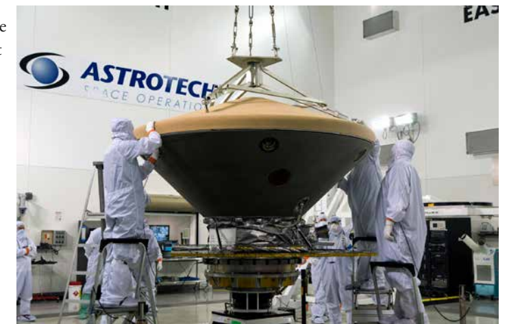
In the Astrotech facility at Vandenberg Air Force Base in California, the heat shield is placed on NASA's Interior Exploration using Seismic Investigations, Geodesy and Heat Transport (InSight) Mars lander on March 29, 2018. Photo credit: USAF 30th Space Wing/Chris Wiant
