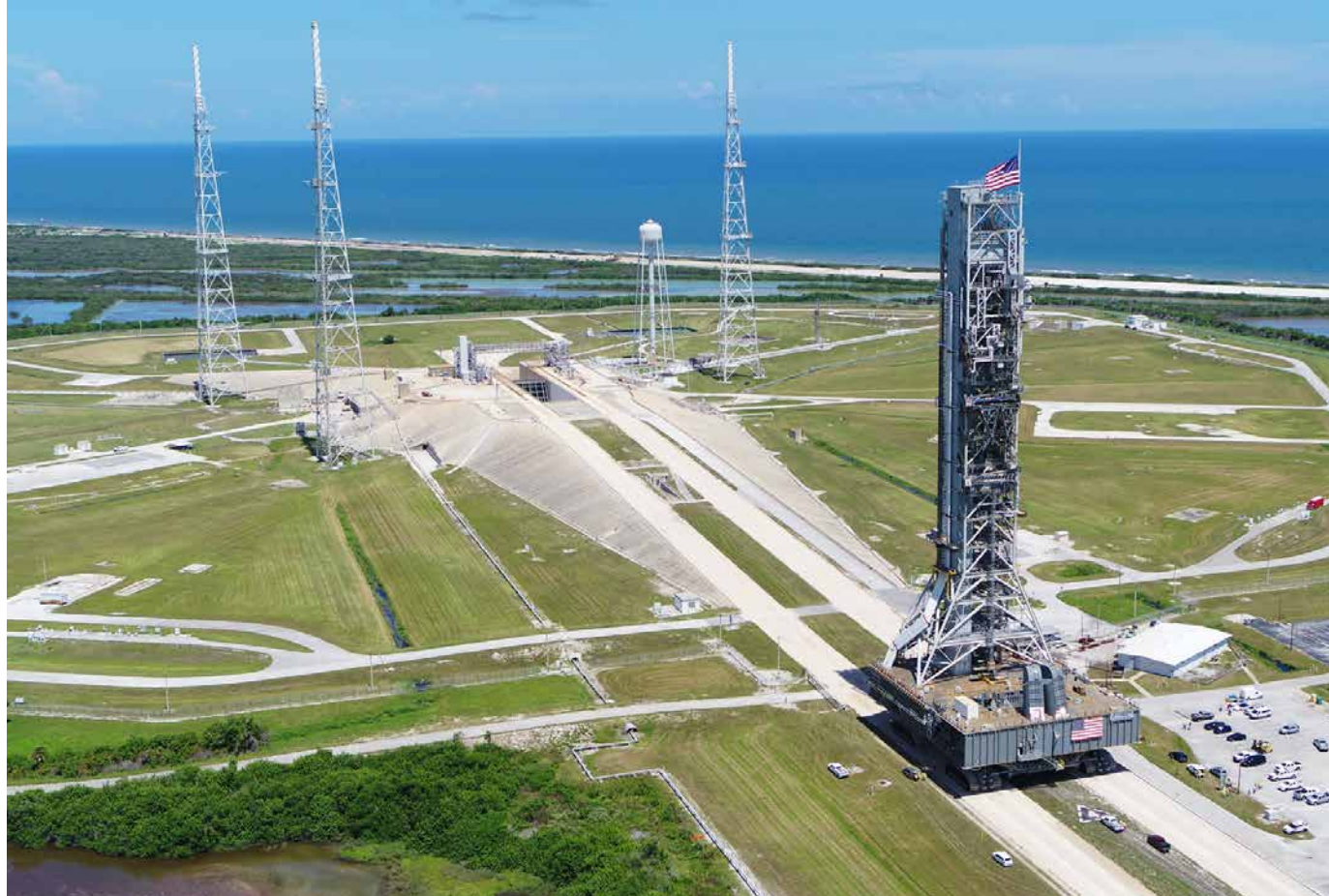
NASA's mobile launcher (ML) atop crawler-transporter 2 arrives at Launch Pad 39B on Aug. 31, 2018, at the agency's Kennedy Space Center in Florida. The ML will undergo a fit check, followed by several days of systems testing. The 380-foot-tall mobile launcher is equipped with the crew access arm and several umbilicals that will provide power, environmental control, pneumatics, communication and electrical connections to NASA's Space Launch System (SLS) and Orion spacecraft. Exploration Ground Systems is preparing the ground systems necessary to launch SLS and Orion on Exploration Mission-1, missions to the Moon and on to Mars. Photo credit: NASA/Jamie Peer
