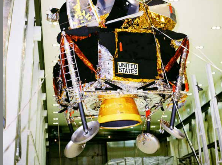
(Above) In the Manned Spacecraft Operations Building (now the Neil Armstrong Operations and Checkout Building) at NASA's Kennedy Space Center in Florida, the lunar module for Apollo 10 is being moved for mating with the spacecraft lunar module adapter. Apollo 10 orbited the Moon in May 1969 and served as a "rehearsal" for the first lunar landing. Photo credit: NASA
