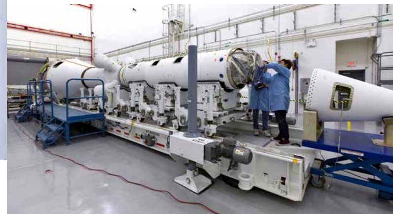
Inside the Launch Abort System Facility (LASF) at NASA's Kennedy Space Center in Florida, workers assemble the Launch Abort System (LAS) on Feb. 5, 2019, that will be used for the Orion Ascent Abort-2 (AA-2) Flight Test. AA-2 is a full-stress test of the LAS, scheduled for Spring 2019. Photo credit: NASA/Kim Shiflett
