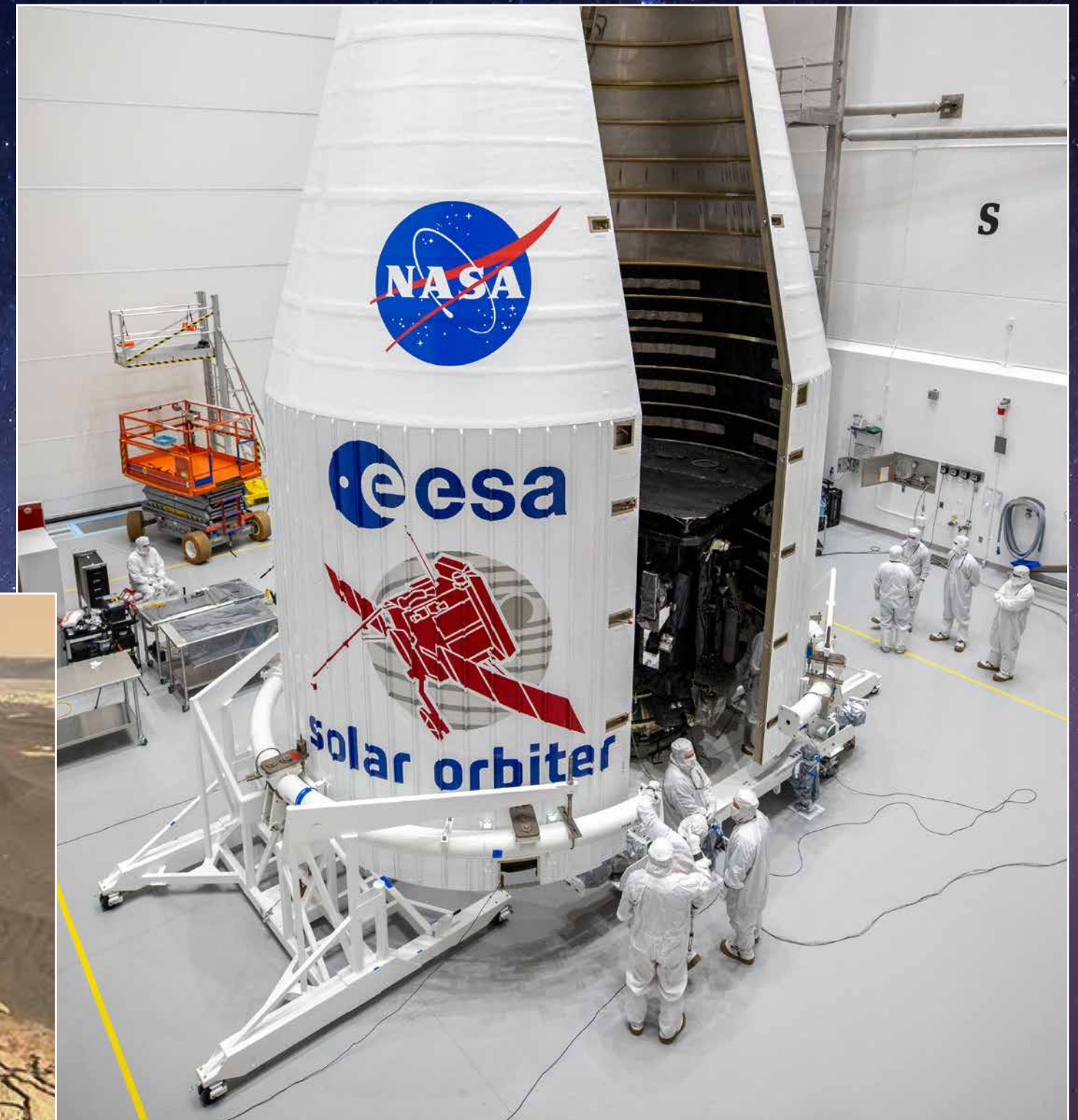
Both halves of a United Launch Alliance Atlas V payload fairing are positioned for installation around the Solar Orbiter spacecraft inside the Astrotech Space Operations facility in Titusville, Florida, on Jan. 20, 2020. The fairing provides a protective, aerodynamic covering to the payload inside during the early minutes of ascent. Solar Orbiter launched aboard the Atlas V rocket from Space Launch Complex 41 at Cape Canaveral Air Force Station in Florida. Liftoff occurred at 11:03 p.m. EST on Feb. 9, 2020. Photo credit: NASA/Ben Smegelsky
