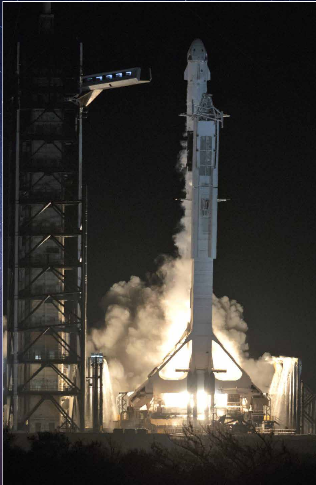
A two-stage SpaceX Falcon 9 rocket lifts off from Launch Complex 39A at NASA's Kennedy Space Center for Demo-1, the first uncrewed mission of the agency's Commercial Crew Program. Liftoff was at 2:49 a.m., March 2, 2019. The SpaceX Crew Dragon's trip to the International Space Station was designed to validate end-to-end systems and capabilities, leading to certification to fly crew. Photo credit: NASA/Kim Shiflett
