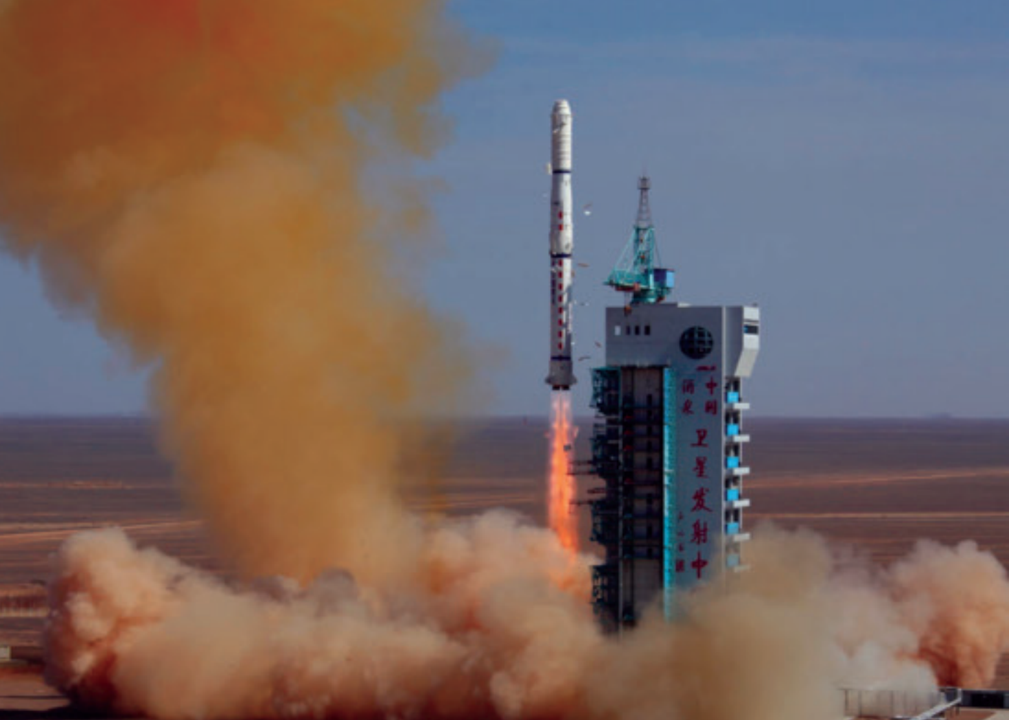
First liftoff from Jiuquan Gobi Desert launch site of the Long March 4C with restartable third stage in late 2010 also marked first launch of three co-orbital Yaogan spacecraft, 9A/B/C, that maneuvered into an ocean surveillance constellation to track U.S. carrier battle groups. Credit: U.S. Naval Institute.
