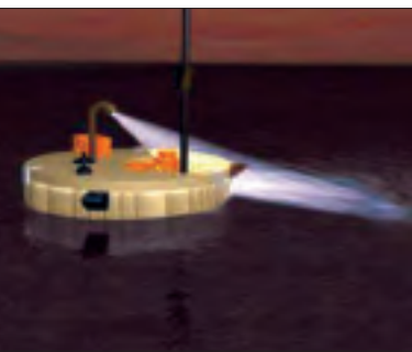
A new $500-million Discovery mission candidate would be this proposed 2016 spacecraft that would fly to Saturn and drop into a large methane lake on the moon Titan. The spacecraft in this graphic uses a floodlight while moving along the surface. The lake lander, developed by Johns Hopkins Applied Physics Laboratory, would compare Titan's characteristics to the hydrological cycle on Earth.
