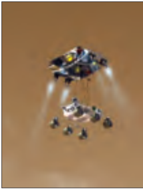
The MAX-C, a new rover for collecting Mars samples, will be lowered by a rocket-powered Sky Crane just like the new Curiosity Mars Science Laboratory being launched in November for landing in late 2012. After MAX-C has completed its mission, another rover, possibly a European one, will also use a Sky Crane landing to collect and load samples into a return rocket.
