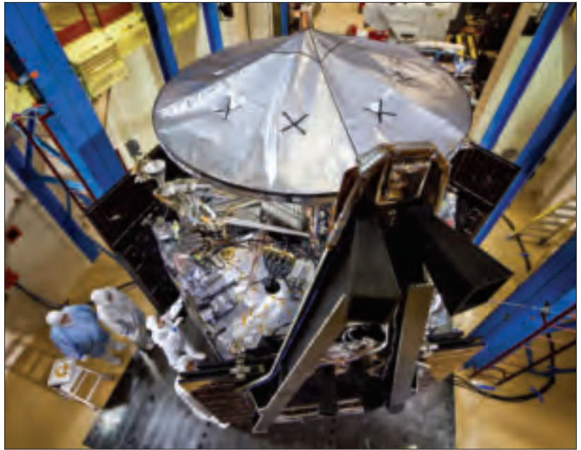
The fully assembled spacecraft went through extensive testing at Lockheed Martin Space Systems near Denver. All three solar array wings can be seen installed and stowed, and the spacecraft’s large high-gain antenna is in place on top. Image credit: NASA/JPL-Caltech/LMSS.
