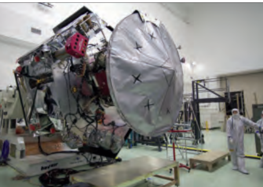
Technicians at the Astrotech payload processing facility in Titusville, Florida, complete installation of Juno's high-gain antenna. Photo credit: NASA/Jack Pfaller.
