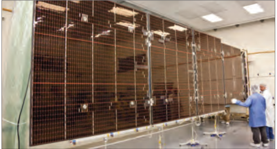
Technicians test the deployment of one of the three massive solar arrays that will power NASA's Juno spacecraft. Image credit: NASA/JPL-Caltech/Lockheed Martin.
