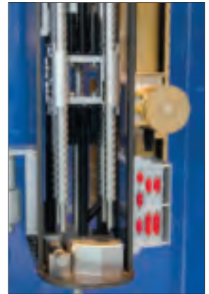
The ExoMars drill will be able to take samples from 2 m below the surface.
