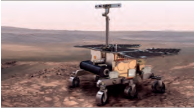
ESA's ExoMars Rover provides key mission capabilities: surface mobility, subsurface drilling and automatic sample collection, processing, and distribution to instruments.
