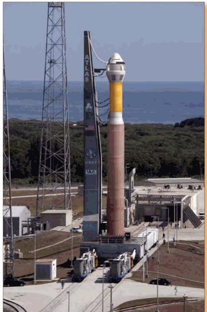
The CST-100 in an artist's rendering. Its two launch abort engines each have a thrust of about 40,000 pounds.
