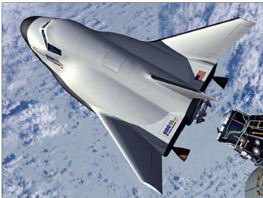
Sierra Nevada's DreamChaser. Its two hybrid abort motors would push the capsule clear of a failing Atlas 5 rocket.
