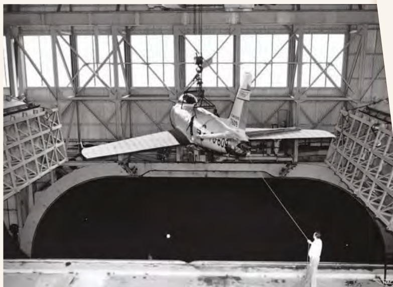
1954 An F-86 aircraft is lowered into the 40x80 Foot Full Scale Wind Tunnel at the NACA Ames Aeronautical Laboratory at Moffett Field, California.
