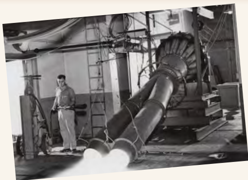
1949 A researcher stands by with a fire extinguisher during research on the effect of twin-jet exhausts inclined toward the ground at the Lewis Flight Propulsion Laboratory. The lab was studying how certain engine installations could decrease an aircraft's takeoff distance.
