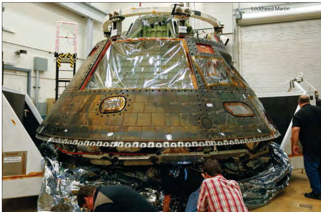
The Orion crew module arrived at Lockheed Martin Space Systems in Littleton, Colorado, after its first exploration test flight in December 2014. The space vehicle's heatshield held up well.
