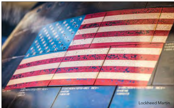
The American flag painted on one of the Orion's thermal protection tiles returned from the first exploration test flight with minor scratches.
