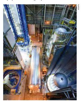
Many components of NASA's Space Launch System, designed to send astronauts to the lunar vicinity in the 2020s, were assembled in preparation for an uncrewed test flight in 2019. The interim cryogenic propulsion stage — the second stage of the SLS and first integrated piece of SLS hardware — was delivered in July to the Space Station Processing Facility at Kennedy Space Center, where it will remain until stacking operations for Exploration Mission 1.
