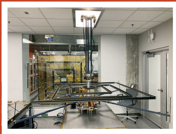
The membrane portion of Caltech's Space Solar Power Demonstrator is deployed in the laboratory prior to its launch in January. Caltech/Momentus
