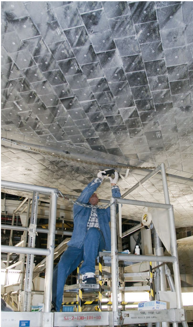
▲ A technician replaces a thermal protection tile on the belly of the space shuttle Atlantis orbiter in preparation for the shuttle program's last flight. Each orbiter is covered in some 30,000 tiles, many of which were replaced after each flight.
