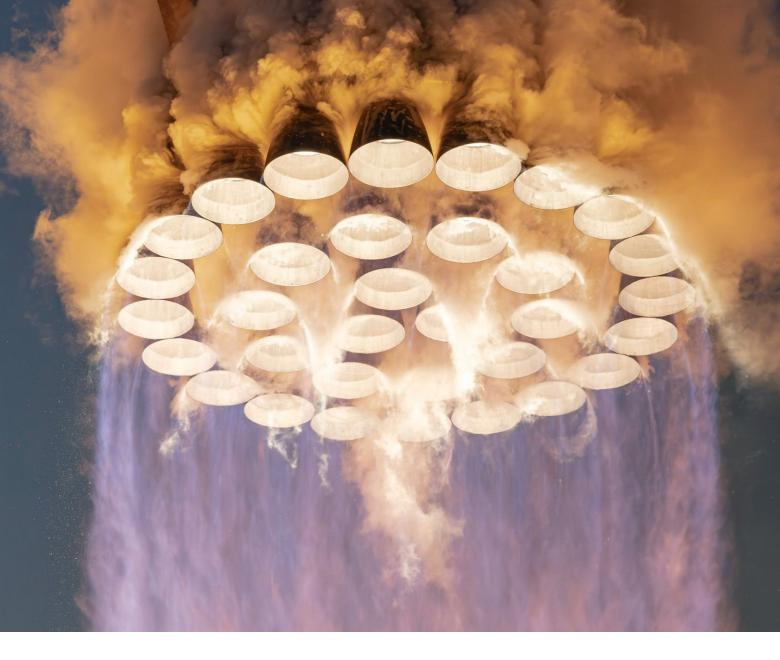
▲ SpaceX built a new kind of conventional engine to power its Starship spacecraft and Super Heavy boosters. Thirty-three Raptors, fueled by liquid methane and liquid oxygen, power each Super Heavy, and six power each Starship.
