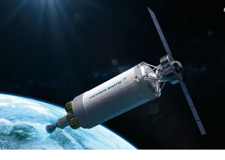
▲ DARPA and NASA believe nuclear thermal propulsion is one option for shortening transit times to Mars. The agencies plan to conduct an in-flight demonstration in 2027, in which a nuclear reactor built by BWX Technologies would heat liquid hydrogen to propel a spacecraft built by Lockheed Martin.
