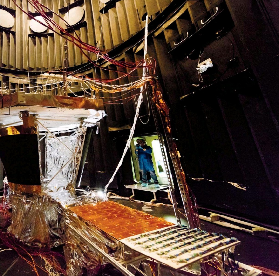
The spacecraft needs a powerful cooling system. This radiator is one of two that will enable the probe to withstand thousands of degrees. Opposite: The mission patch.
