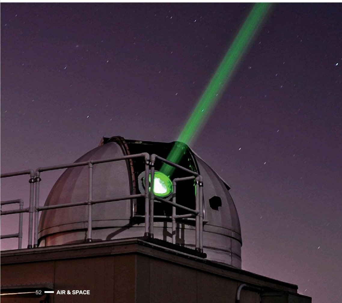
← NASA's Next Generation Satellite Laser Ranging System fires a beam into the sky over the Goddard Space Flight Center in suburban Washington, D.C.
