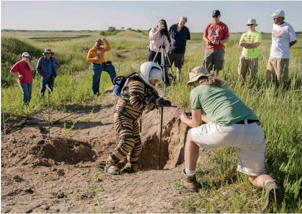
← Spacesuit designers at the University of North Dakota test their experimental NDX-1 model in the field in 2009. Modest NASA-funded research like this has yielded interesting results, but not a finished, flight-ready suit.
