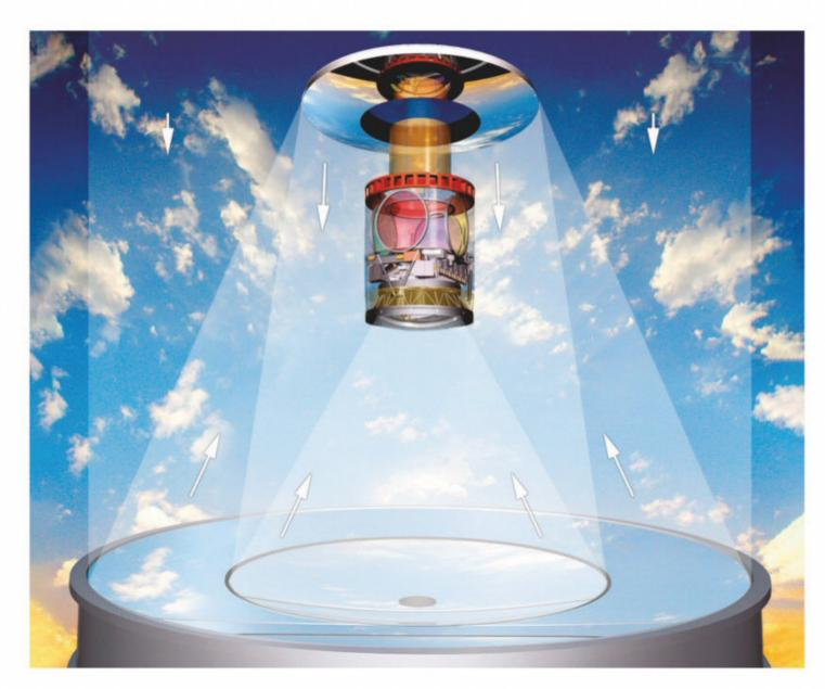
Light streaming down from distant stars and galaxies hits the large primary mirror, bounces up to a curved secondary mirror, back down to a third mirror set inside the primary (sharing the same piece of glass), then finally back up to the telescope's three-ton camera. images of an object-the universe in time-lapse.
