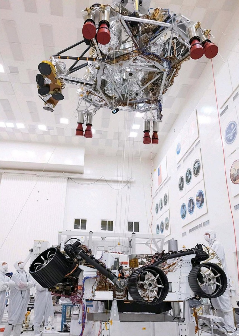
↑ Jet Propulsion Laboratory tests the sky crane descent system, which will gently lower Mars 2020 to the Red Planet's surface. The same method successfully landed Curiosity in 2012.
