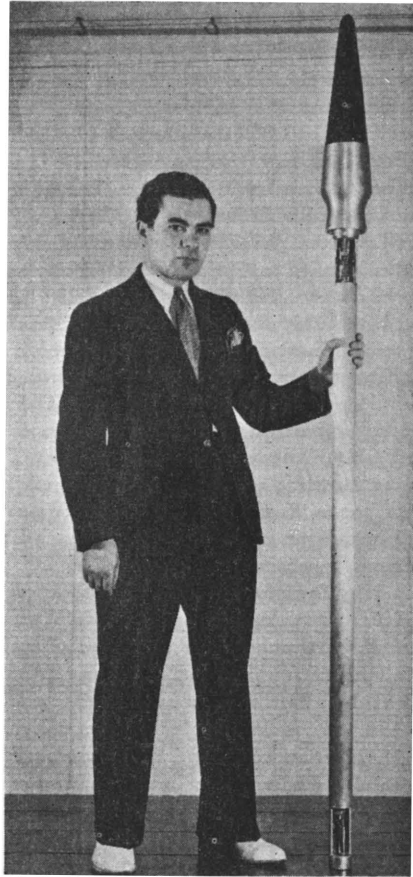
Mr. Lent with the motor and upper tank of his rocket. Complete, it will be twice the length indicated here.
