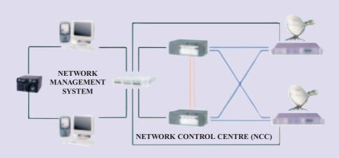
Channel Satellite Terminal (RCST) provides terminal access to the satellite. The NMC handles the system configuration and manages the AmerHis network elements, supporting remote configuration and monitoring of the NCC, user terminals, gateways and OBP, as well as providing fault, configuration, performance and security features for all elements.
