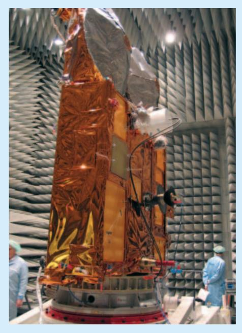
On the payload side, after its arrival at IABG, the electronics of the SIRAL altimeter developed by Alcatel (F) have been mated with the double antenna manufactured by Saab (S), and successfully tested. The integration on the spacecraft has taken place in a timely manner and the altimeter's performance figures are nominal. Following this test, the CryoSat satellite has been moved to a dedicated IABG facility to undergo a first series of electromagnetic-compatibility tests.
