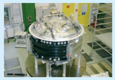
The qualification models of the Herschel scientific instruments have successfully completed their functional and performance testing and have been delivered to industry for integration into the test cryostat. Also, the Planck HFI qualification-model instrument has been delivered to Alcatel for integration with a LFI dummy and into the Planck Payload Module qualification model.
