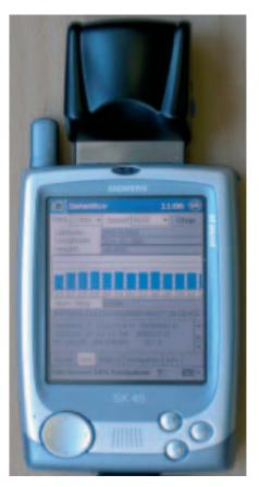
During field testing in Finland, the new receiver delivered horizontal positioning accuracies of 1-2 metres and vertical accuracies of 2-3 metres. In a further step, the device has been integrated into a Siemens SX45 mobile phone.
