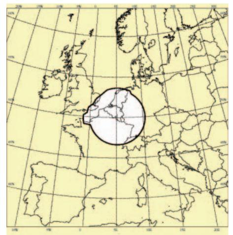
A typical coordination contour, in this case for SMART-1 mission support from ESA's Redu station in Belgium
