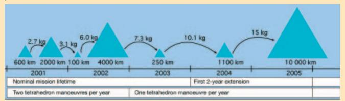
The triangles show schematically the size of separation distances of the four Cluster satellites, with the actual separation distances in kilometres given below the triangles. The masses show how much fuel was consumed during the manoeuvres conducted for each new tetrahedron constellation (Courtesy of D. Sieg, ESOC)
