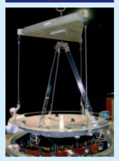
Optical/structural/thermal model of the ADM-Aeolus telescope being mounted on the instrument
