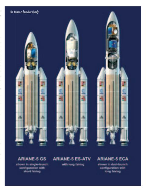
launcher is protected by a payload fairing during the atmospheric flight phases. It is a lightweight carbon-sandwich structure and is produced in three lengths to accommodate different sizes of payloads. The fairing length may be further increased in height by adding cylindrical sections (Adaptateur Cylindrique, or ACY).
