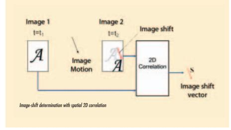
The optical-processor model consists of an optical unit and an electronic module. It processes two standard video signals from the camera's matrix sensors and produces the real-time image-motion record. The optical unit uses standard video cameras as image sensors for the same reason as the camera. This limits the image processing rate to 30 optical Fourier transforms per second, or 15 correlations per second per optical Fourier processor (one correlation
