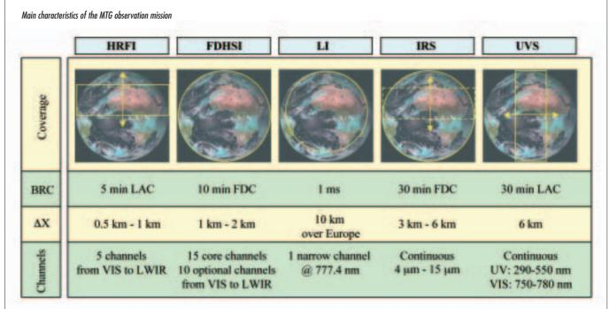
BRC: Baseline Repeat Cycle FDC: Full Disk Coverage LAC: Local Area Coverage (18° x 6°)  $\Delta X$ : Spatial resolution UV: ultraviolet VIS: visible LWIR: longwave infrared
