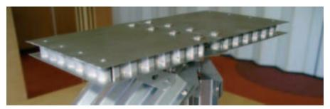
Reusable rudder metallic structure building-block element (Courtesy of Dutch Space)
