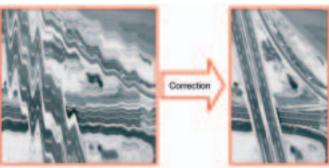
Examples of SmartScan image correction on the basis of imagemotion records
