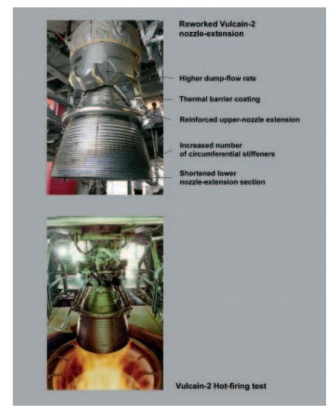
The Vulcain-2 engine and its major modifications after completion of the reworking activities conducted in the framework of the Ariane Recovery Plan
