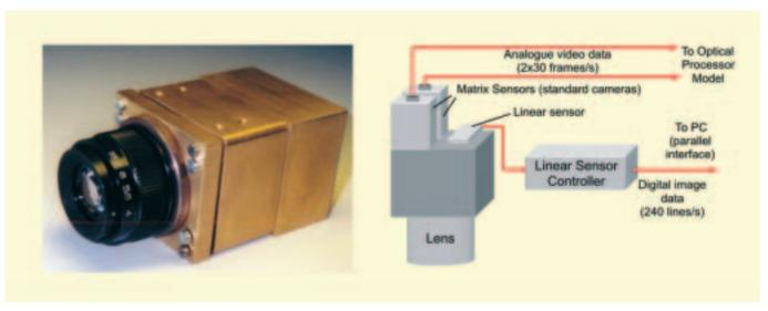
The breadboard model of the SmartScan pushbroom camera
