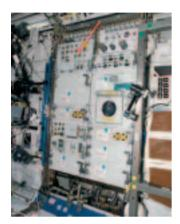
Housed within the Human Research Facility #2, the Pulmonary Function System installed in the ISS's Destiny laboratory
