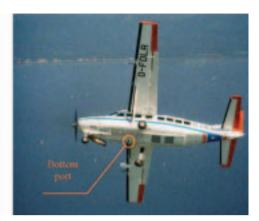
The SmartScan airborne flight-test configuration
