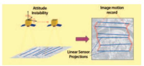
Image distortions due to satellite attitude instability while scanning with a linear image sensor
