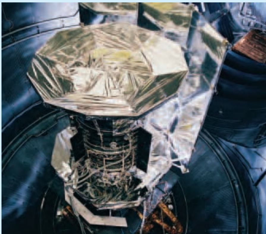
The Herschel spacecraft in the Large Space Simulation (LSS) facility at ESTEC (NL) for the cryogenic lifetime test
