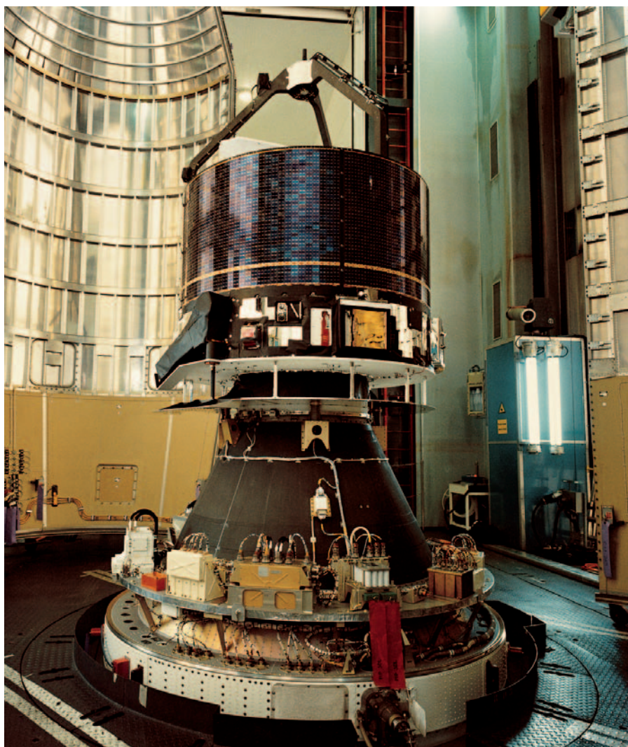
The Giotto spacecraft installed on its Ariane-1 launcher in Kourou, French Guiana
