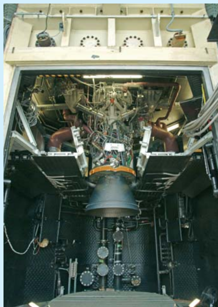
The Expander Demonstrator rocket engine on its test stand at DLR's test facilities in Lampholdshausen, Germany
