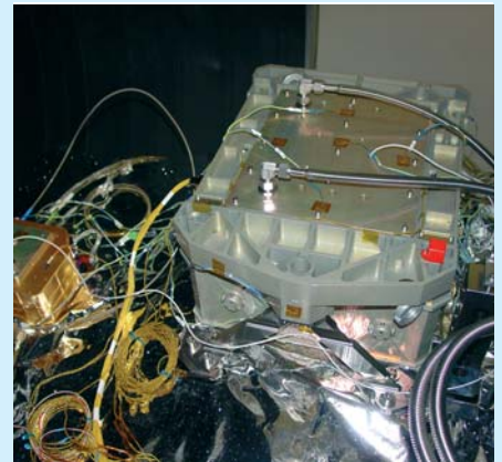
ALADIN laser assembly in vacuum test configuration
