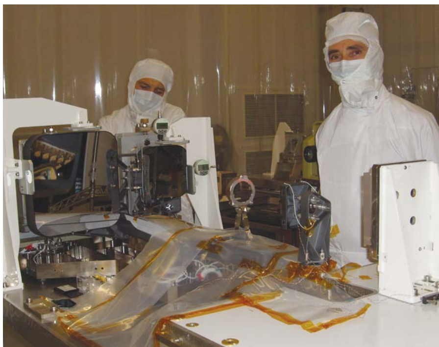
The qualification model of the NIRSpec front optical system undergoing testing (Sagem)
