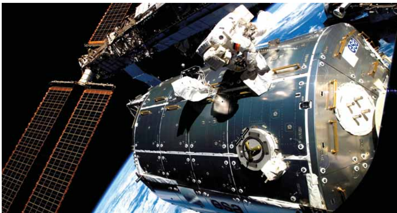
Floating near Columbus, Hans Schlegel makes his first-ever spacewalk outside the ISS, the second spacewalk of the STS-122 mission, lasting six hours 45 minutes. Schlegel and NASA astronaut Rex Walheim made the spacewalk to replace a nitrogen tank used to pressurise the Station's ammonia cooling system
