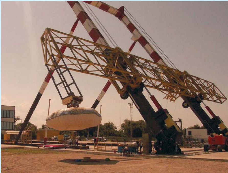
Technology developments crucial to Enhanced ExoMars have been made, such as tests of Vented Airbags
