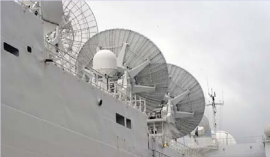
The Armor C-band radars on the French naval vessel Monge (DGA)
