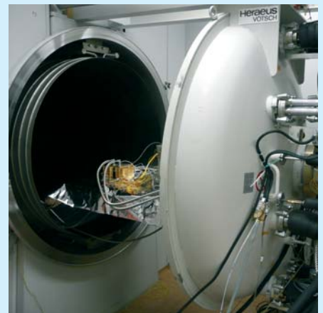
Transmitter laser assembly integrated in the thermal vacuum chamber
