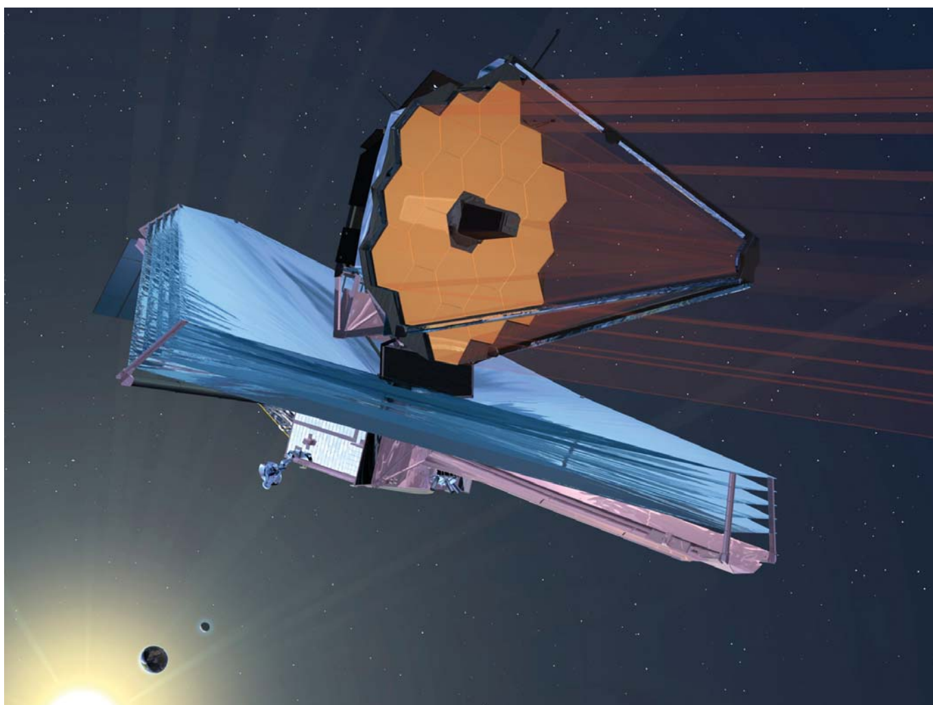
Artist impression of the deployed JWST in orbit showing the 6.55 m segmented telescope mirror and matching sunshade (Northrop-Grumman)
